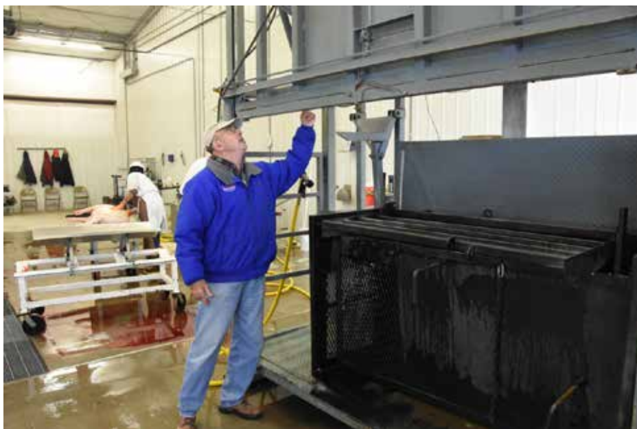
Above: inside the docking unit: Mike Callicrate checking 'kill box'; below and bottom: 'kill box' (adjustable size for big/small animals)
